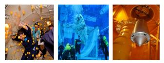
Figure 2. Methods to simulate low-gravity conditions include use of parabolic flight (left), neutral buoyancy in large water tanks (center) and use of drop towers (right).
