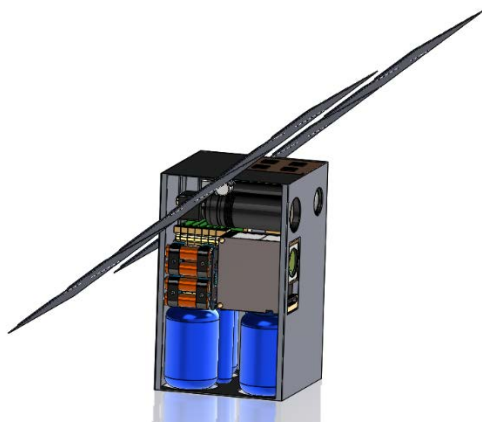
Fig. 3. LOGIC X utilizes a 12U bus and enhanced zoom lens providing up to 200x magnification for both the visible and thermal imager and nearly 3 times the fuel of LOGIC.
