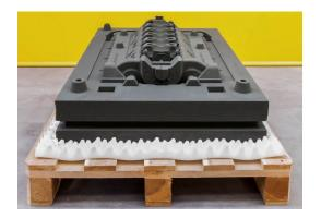
Fig. 3. ExOne® BJ printed sand mold for metal casting.
