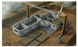
Fig. 4. Contour Crafting architectural scale printer [7].
