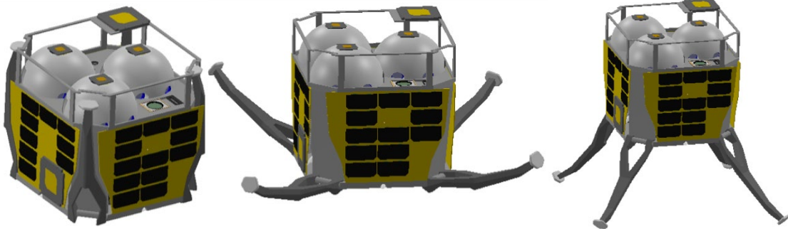
Fig. 4. Sequence of deployment of the landing legs.
