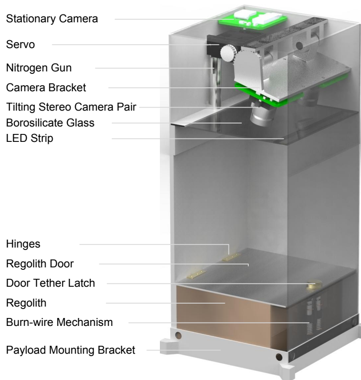
Figure 3: Illustration of scientific payload design oriented with sealed regolith chamber on the bottom and all instrumentation protected behind borosilicate at top.
