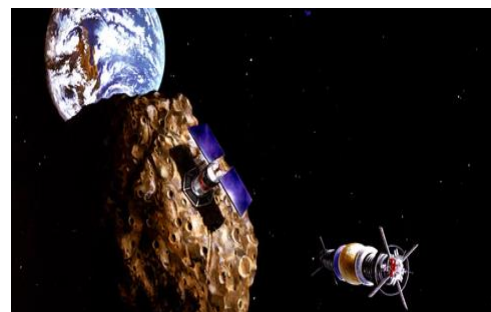
Fig. 1. Water extracted from asteroids and small bodies can be readily used as fuel in a solar thermal steam propulsion system (courtesy NASA).
