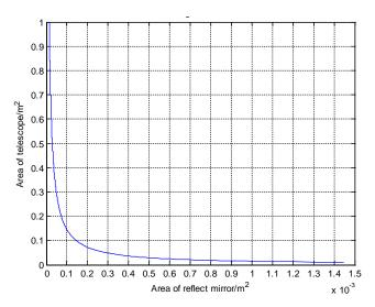
Figure 5: Size of telescope required to detect signal from a reflector mirror in LEO.
