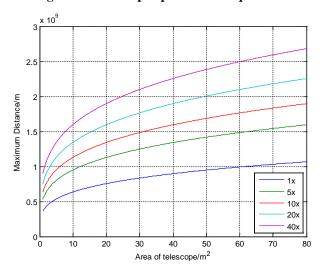
Figure 8: Max comms. distance for telescope/reflector.
