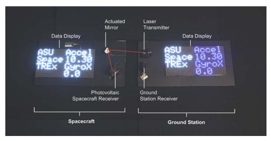
Figure 10: Photo of benchtop system in operation.
