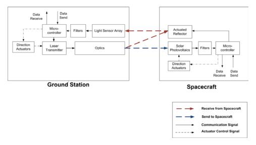
Figure 2: Extensible Laser Communication System Architecture
