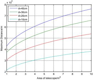
Figure 7: Maximum communication distance achieved for telescope and reflector mirror combination.
