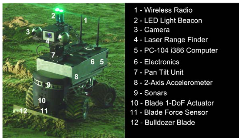
Figure 26: An Argo robot equipped with a 1 DoF bulldozer blade, a laser range finder, a pair of Logitech ® Quickcams TM affixed to the pan-tilt unit and an assortments of other sensors.
